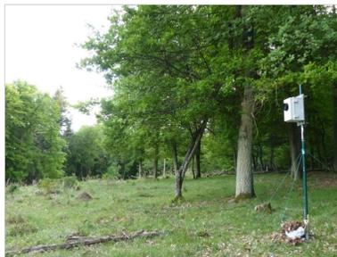
Fig. 3: Batcorder in a gap in woodland.
